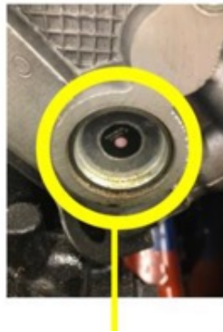
Overheated Pink Sensor 255°F Coolant Temp
